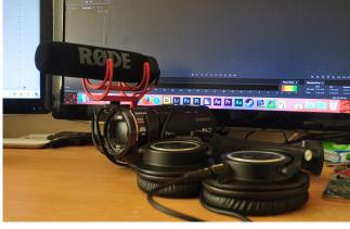
The RODE VideoMic GO's Specifications. It has a hypercardioid polar pattern meaning it picks up less of the reverb from the sides and behind and more of the direct sound from the front. It also has a limited frequency response, 100Hz - 16kHz. This means it is less susceptible to any bass frequencies and any higher pitched frequencies. This is good for recording my vocal speech as it limits to the vocal range, but not quite as harsh at the 3kHz telephone band.
