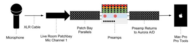
One benefit of this method is that you are getting the exact same signal from the microphone with zero latency to each of the pre-amps. It is also quite simple to set up once you have made sure it is safe to do so. As this is all done in the analogue realm, there are no extra analogue to digital conversions or digital duplication of signals.
