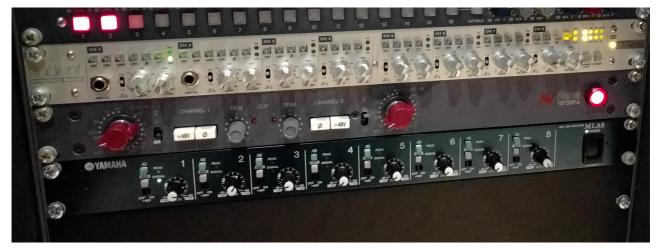
As the parallel is effectively connecting all the cables together, you only need to feed phantom power from ONE of the pre-amps. Applying phantom power to unbalanced
